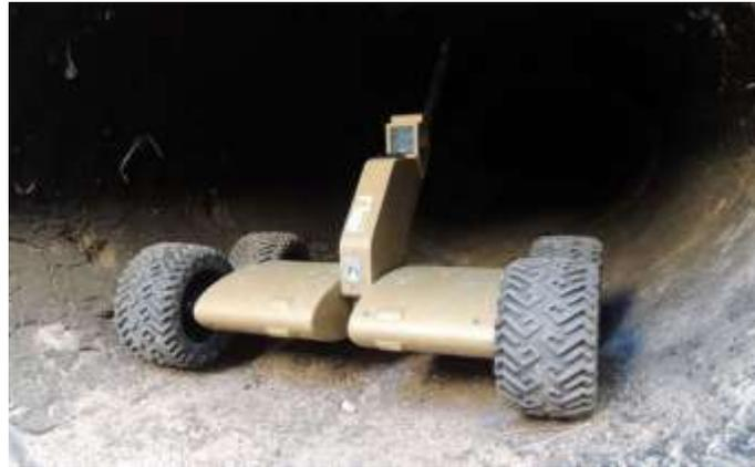
Another robot adapted for tunnel surveillance is the Pointman Small UGV (SUGV). According to ARA over 50 Pointman Tactical Robots are already deployed with police, SWAT, government and first responder teams across the United States. This wheeled robot, built by ARA is currently has recently been used in tunnel detection, operating around Nogales, on the Arizona border.
