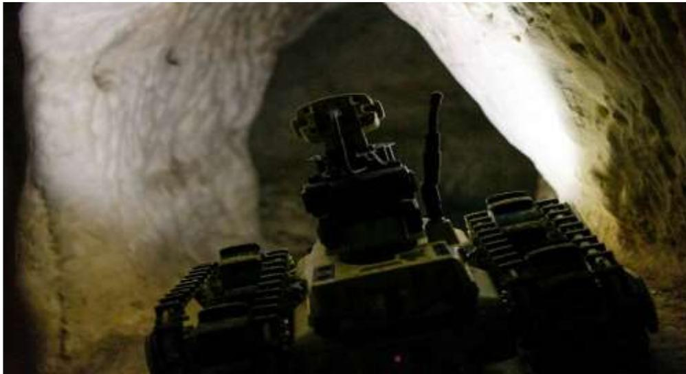
Operating robots within the confined space of the tunnel is quite a challenge, as remotely controlled robots must deliver effective orientation beyond line of sight. Wireless communication with the robot is another issue requiring deployment of repeaters to extend its range. Orientation without GPS is also a challenge, which can be solved by mapping the subterranean space, although this process may require time.
